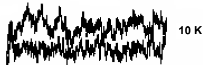
Fig. 8. Josephson hysteresis loop for the sample in Fig. 7: MMMA signal versus magnetic field from -40G to 40G.
