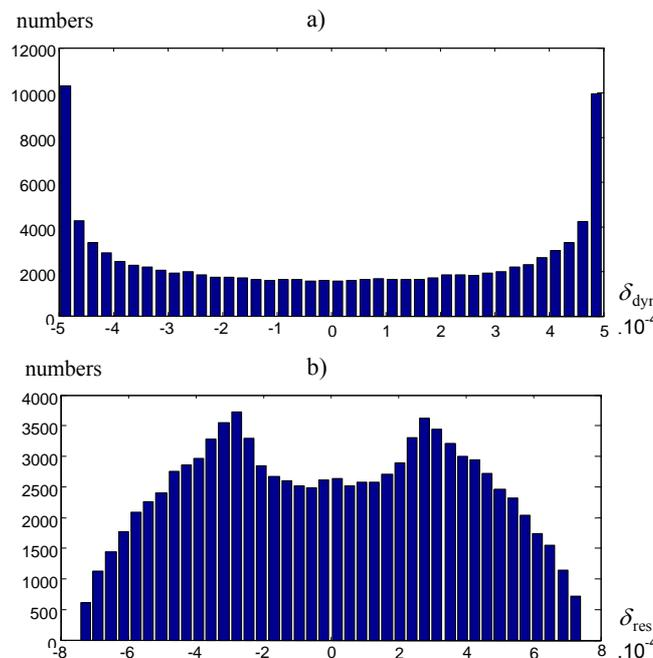
Fig. 10. Exemplary histograms: a) amplifier dynamic error, b) resultant error composed of dynamic and quantization error.
