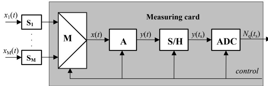
Fig. 1. Basic scheme of measurements in a system.
