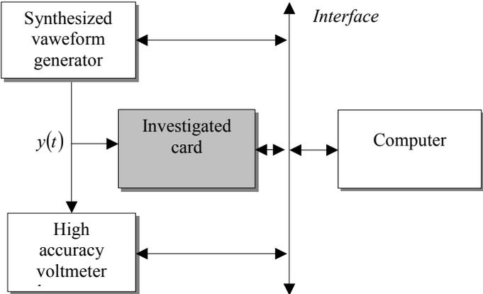
Fig. 7. System for identification of the measuring card errors.
