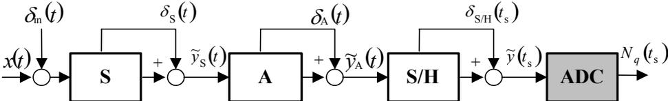
Fig. 6. Propagation of the input signal in the system measuring chain.
