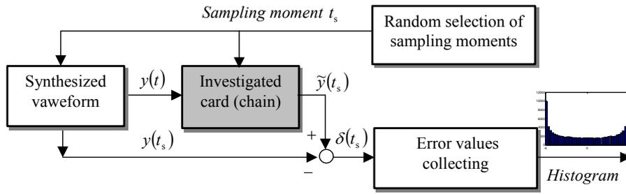
Fig. 8. Scheme of procedure of error value set determination.
