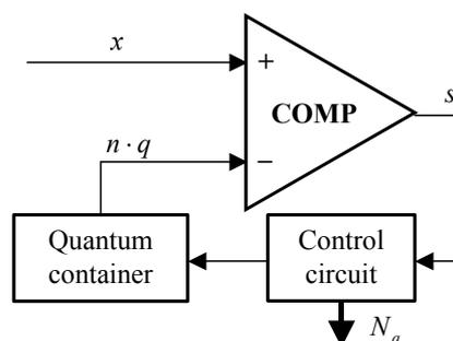
Fig. 2. Basic scheme of a quantizer.
