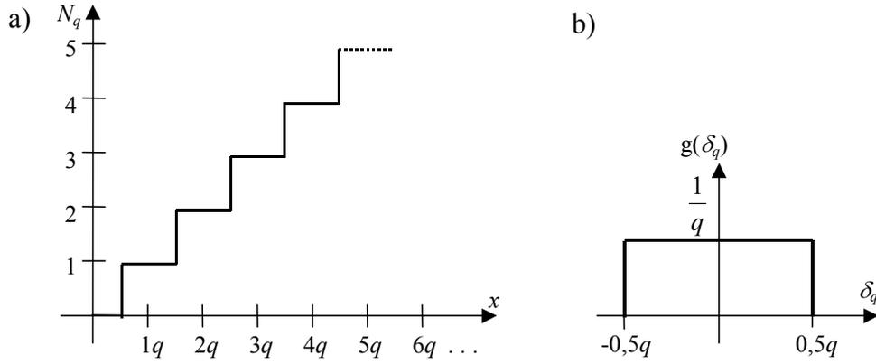
Fig. 5. a) Characteristic of the quantizer described by Eq. (11), b) distribution of its quantization error.
