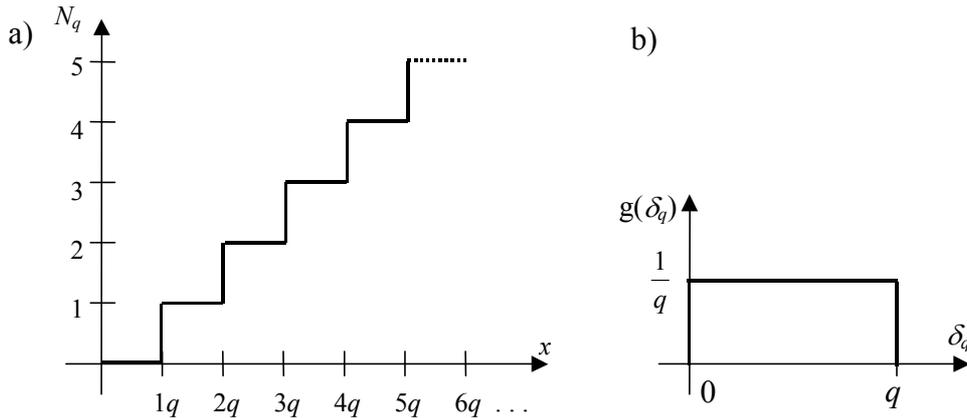
Fig. 4. a) Characteristic of the quantizer, b) distribution of the quantization error.
