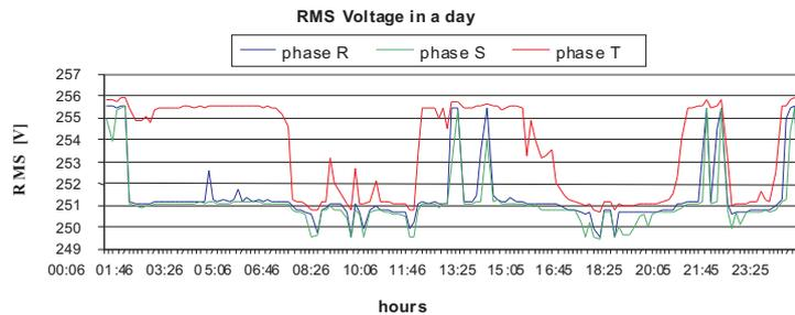
Fig. 6b. Three phase RMS voltage monitoring in a day.
