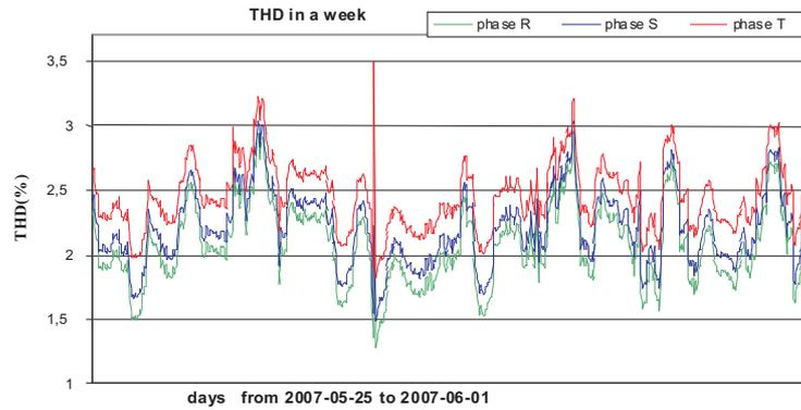
Fig. 5a. Three phase THD voltage monitoring in a week.
