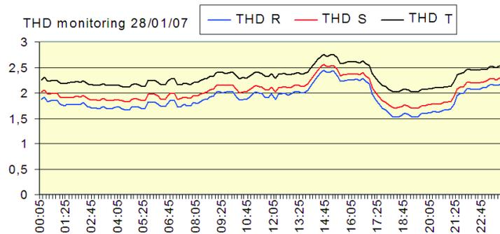
Fig. 5b. Three phase THD voltage monitoring in a day.
