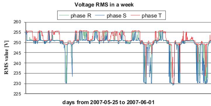
Fig. 6a. Three-phase RMS voltage monitoring in a week.
