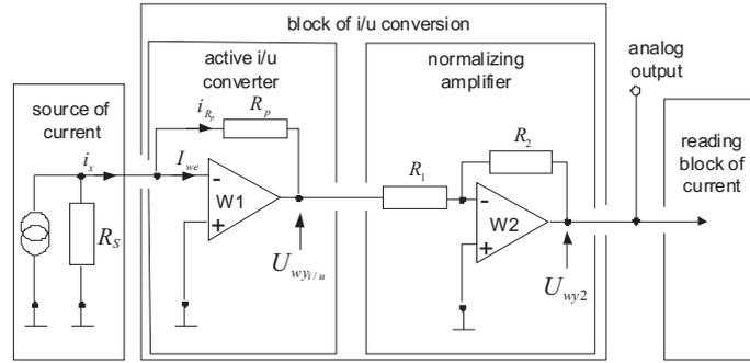
Fig. 4. Schematic of the picoammeter with an active i/u converter.
