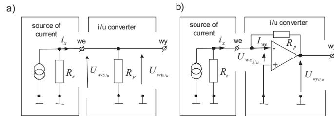
Fig. 2. Circuits of analog i/u conversion: a) passive i/u converter, b) active i/u converter.
