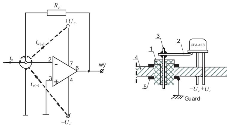
Fig. 6. Leakage currents in the insulating material of the epoxy printed circuit board: a) leakage tracks between input and supply connections, b) method of elimination of current-generating phenomena:
