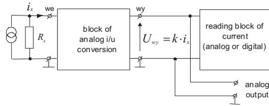
Fig. 1. Block diagram of a picoammeter with analog i/u conversion.
