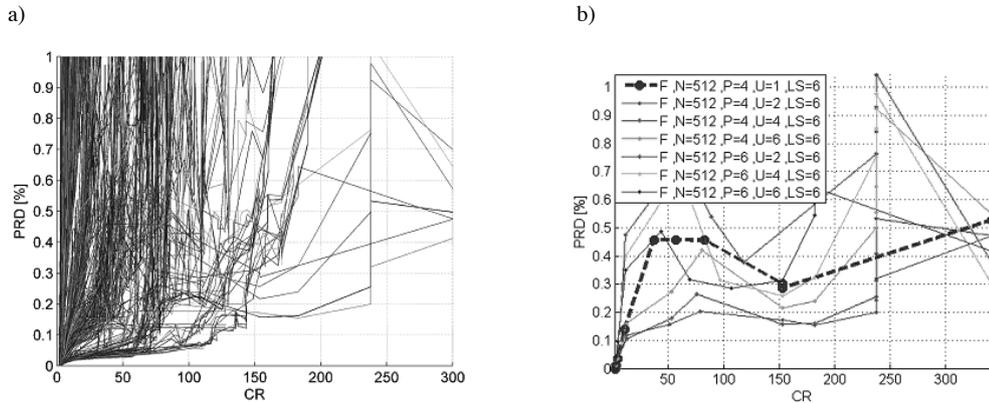
Fig. 5. a) Compression results for all configurations in brute force testing method (3072 curves), b) Best compression results selected for signal  $F$  (see Fig. 4) in the legend the length of the frame  $N$ , length of  $P$  and  $U$  filters and the number of lifting decomposition stages  $LS$  are given.
