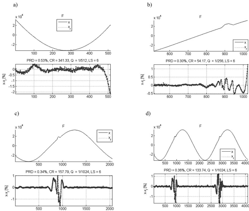
Fig. 6. Best compression results obtained for test signal  $F$  from Fig. 4,  $P = [-1/16, 9/16, 9/16, -1/16]$ ,  $U = [1/2]$ , a)  $N = 512$  first frame, b)  $N = 512$  second frame, c)  $N = 2048$ , d)  $N = 4096$ . The compression results are given in lower subplot titles. In all cases signals  $x$  and  $x_r$  (upper subplots) and their difference (lower subplots) are shown.
