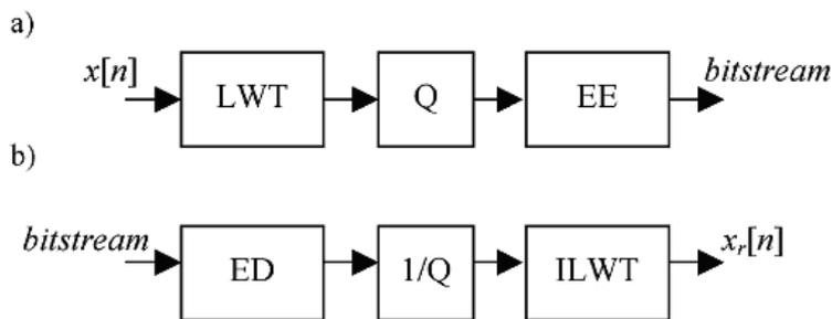
Fig. 1. Compression algorithm a) encoding, b) decoding, denotations:  $x[n]$  – input signal,  $x_r[n]$  – reconstructed signal, LWT – integer Lifting Wavelet Transform, ILWT – Inverse integer Lifting Wavelet Transform, EE – Entropy Encoder, ED – Entropy Decoder,  $Q$  – quantization  $0 < Q \leq 1$ .
