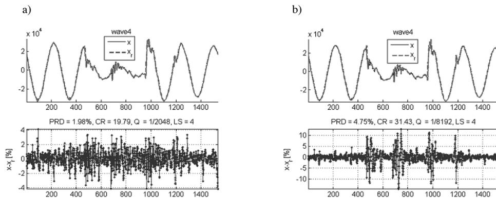
Fig. 9. Compression results for signal *wave4*; original signal  $x$ , reconstructed signal  $x_r$  and the difference between these signals is shown for: a) CR = 19.79, PRD = 1.98% and b) CR = 31.43, PRD = 4.75%.
