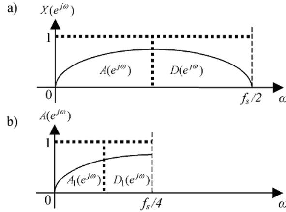
Fig. 3. Frequency interpretation of Mallat decomposition. Spectra of discrete signals are shown in the range from 0 to  $f_s/2$  Hz. Denotations consistent with Fig. 2,  $f_s$  – sampling frequency: a) first decomposition level, b) second decomposition level.
