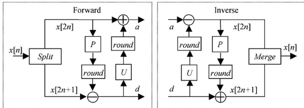
Fig. 2. Integer LWT computations:  $x[n]$  – input signal – length  $N$ ,  $a$  – approximation coefficients length –  $N/2$ ,  $d$  – detail coefficients length –  $N/2$ .
