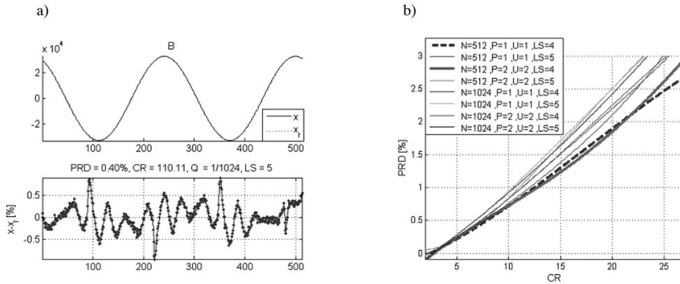
Fig. 8. a) Compression results for signal *B*. b) Averaged compression results for test signals (Fig. 4) except signals *B*, *E* and *F*.
