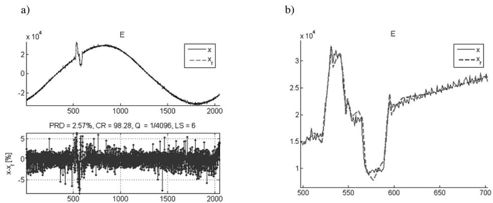
Fig. 7. Compression results for signal  $E$ : a) original signal  $x$ , reconstructed signal  $x_r$  and the difference between these signals, b) detailed view of the transient disturbance in original  $x$  and reconstructed  $x_r$  signals.
