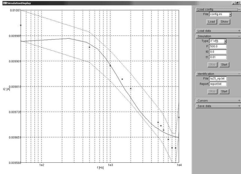
Fig. 4. Bode characteristics of electronic current transducer obtained for extracted values of the parameters.
