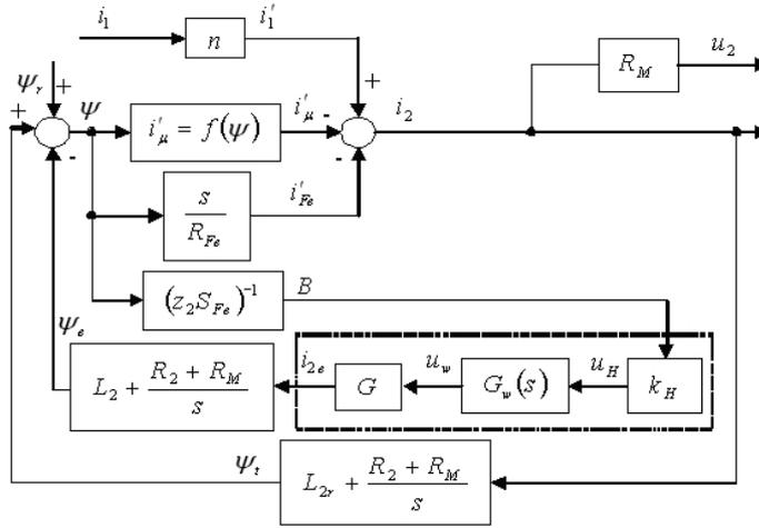
Fig. 2. A block diagram of the electronic current transducer model [11].
