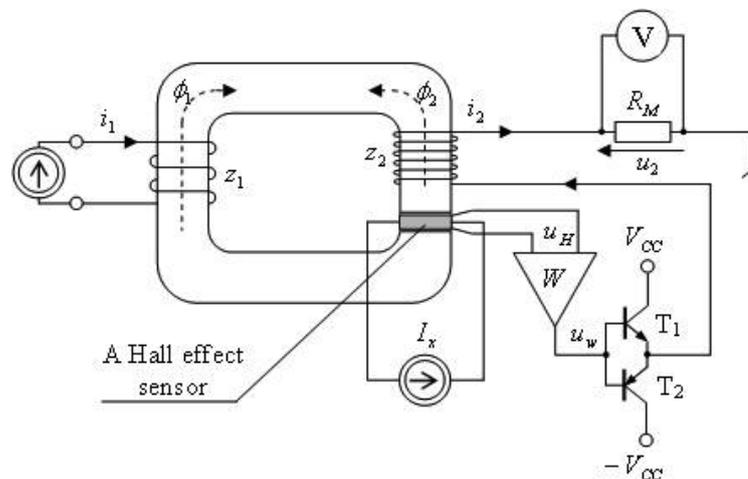
Fig. 1. A visual diagram of the electronic current transducer with a Hall effect sensor in the negative feedback loop.
