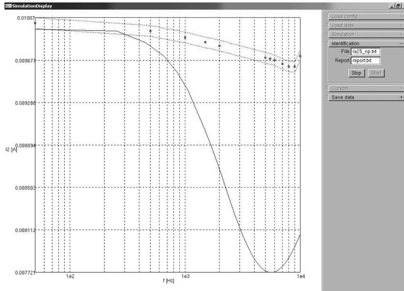
Fig. 3. Bode characteristics of electronic current transducer obtained for the first trial values of the parameters.
