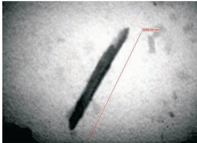
Fig. 4. TEM image of an electrodeposited nanowire.
