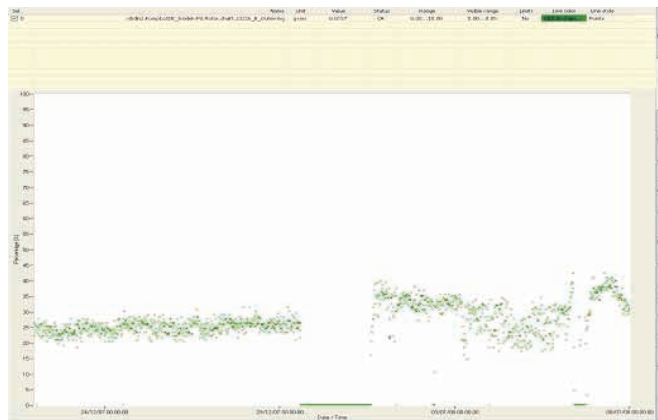
Fig. 9. Trend of the energy in the band in the envelope order spectrum, calculated around the 8.34X (outerring ball pass).
