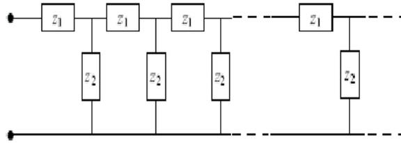
Fig. 4. Equivalent radiotechnical scheme of the nonstationary structure of the layer of a composite material:  $z_1$  – inductive component of the impedance;  $z_2$  – capacitive component of the impedance.
