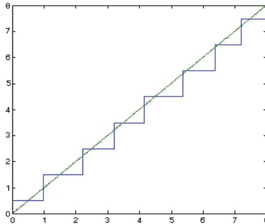
Fig. 4. Characteristic of exemplary 3 bit A/D converter with quanta burdened distortion errors.
