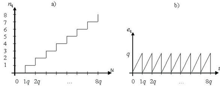
Fig. 2. Exemplary 3 bit quantizer, (a) characteristic, (b) quantization error.
