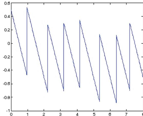
Fig. 5. Total error of exemplary 3 bit A/D converter.
