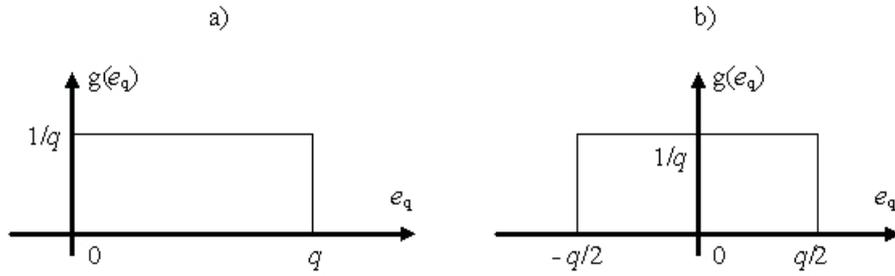
Fig. 3. Distributions of a quantization error, (a) for the quantizer with the characteristic shown in Fig. 2a, (b) for the quantizer after correction of the systematic component of a quantization error.
