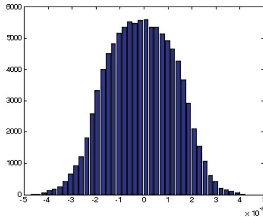
Fig. 8. Histogram of the total error of 8 bit A/D converter with relative quantum distortion  $d = 3\%$ .
