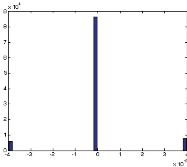
Fig. 7. Standard error histogram of exemplary 8 bit flash A/D converter.
