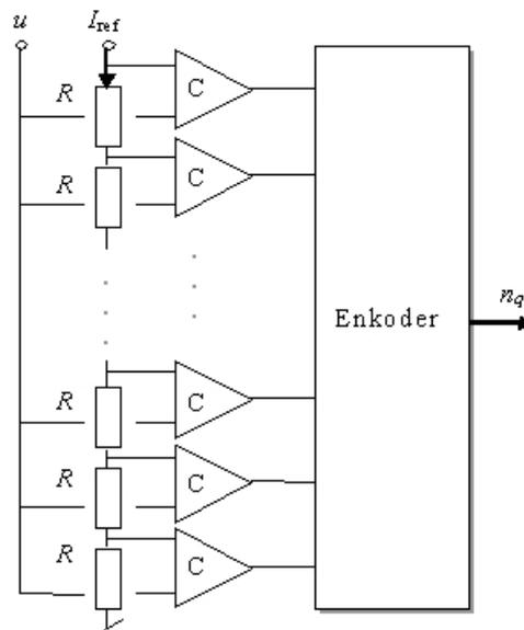
Fig. 1. Scheme of flash A/D converter.
