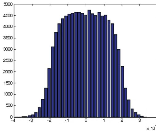
Fig. 9. Histogram of total error of exemplary 8 bit A/D converter after adjustment, relative quantum distortion  $d = 3\%$ .
