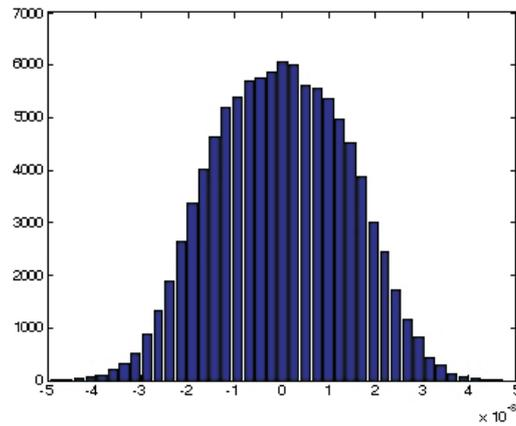
Fig. 10. Histogram of total error of exemplary 8 bit A/D converter, relative distortion  $r = 3\%$ , standard deviation of the noise error with normal distribution  $\sigma = 0,1q_{\text{nom}}$ .
