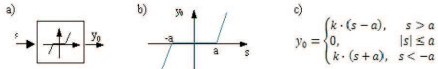
Fig. 2. Converter with characteristic with dead zone: a) symbol, b) input-output characteristic, c) processing equation.
