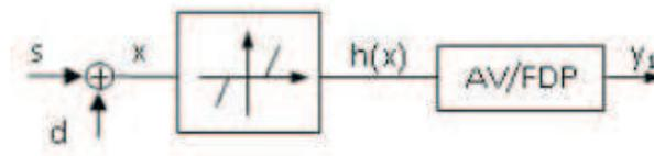
Fig. 5. Linearization of converter characteristic with a dither signal.
