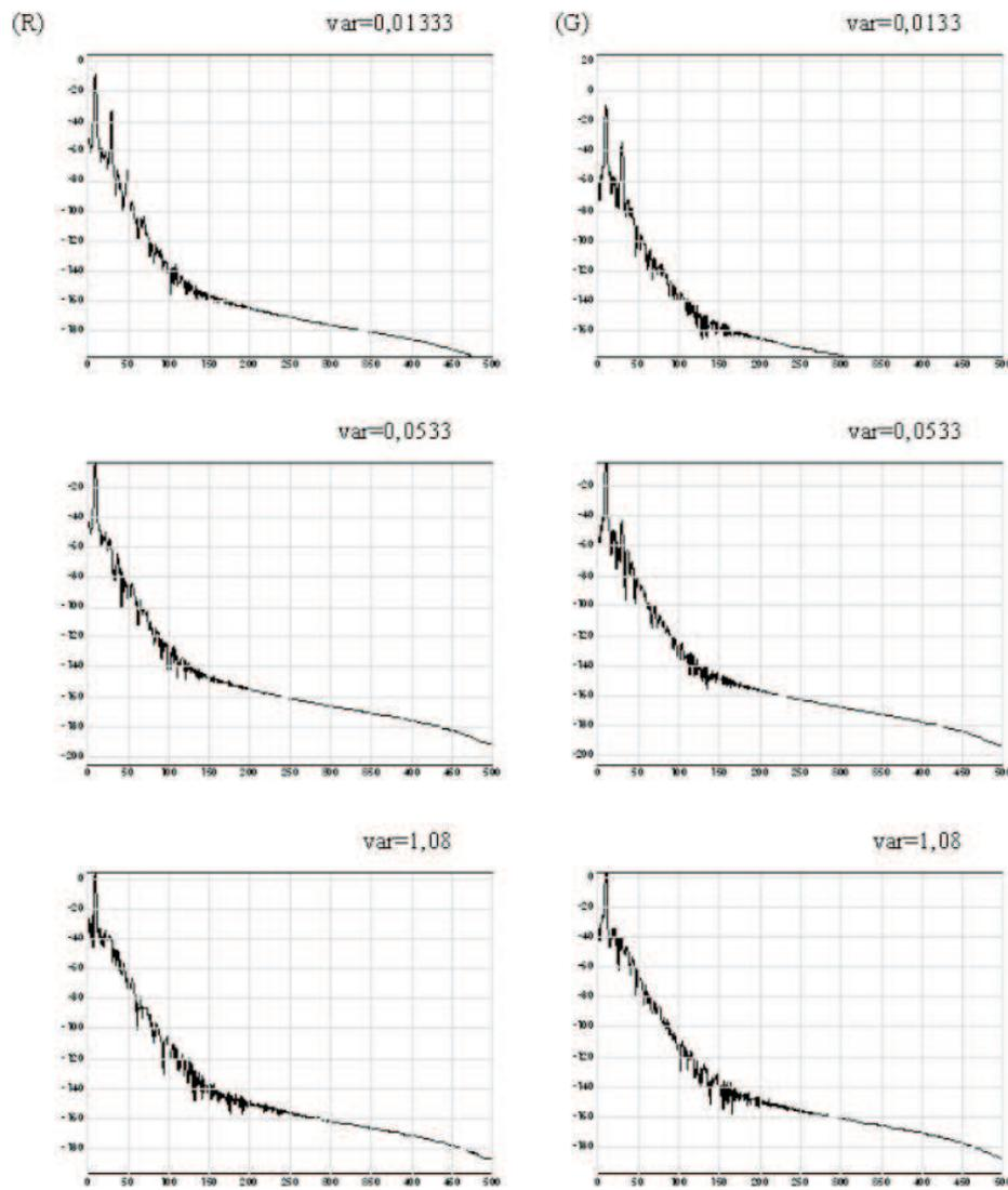
Fig. 8. Spectrum of the converter output signal,  $-0.2 \leq DZ \leq 0.2$   $A = 0.18$ : column (R) – dither with rectangular PDF, column (G) – dither with gaussian PDF.
