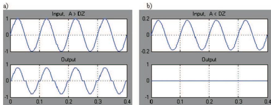
Fig. 3. Input and output signal of the converter,  $-0.2 \leq DZ \leq 0.2$ , a)  $A = 1$ , b)  $A = 0.18$ .
