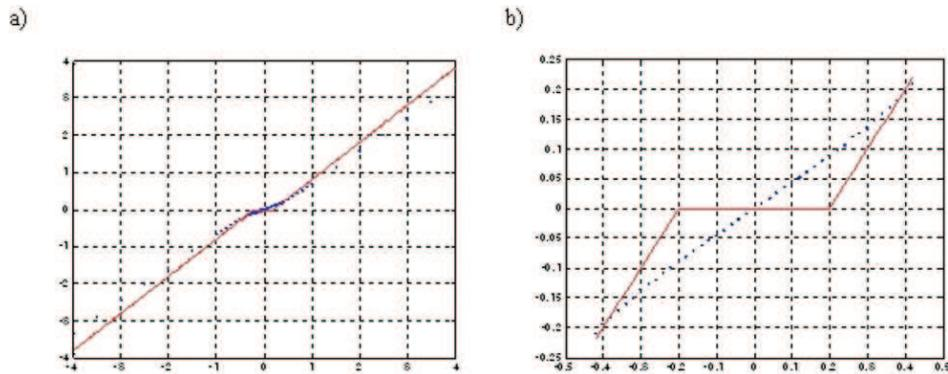
Fig. 7. Characteristic of a converter with dither: a) whole, b) fragment.
