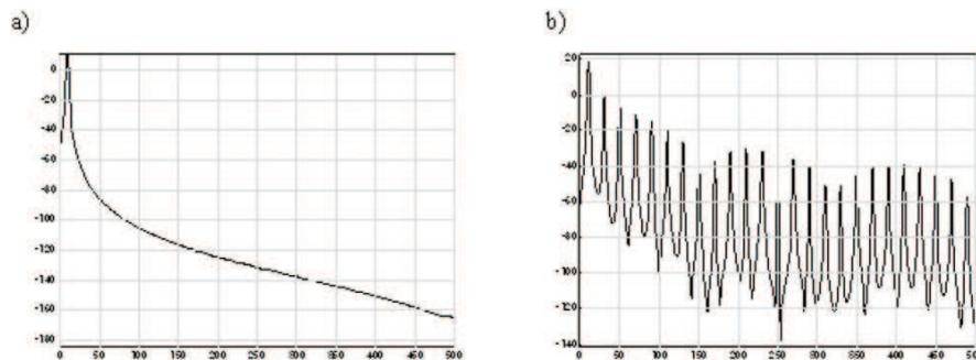
Fig. 4. Converter with dead zone: a) spectrum of input signal, b) spectrum of output signal.
