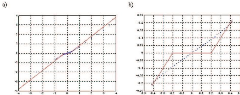
Fig. 7. Characteristic of a converter with dither: a) whole, b) fragment.
