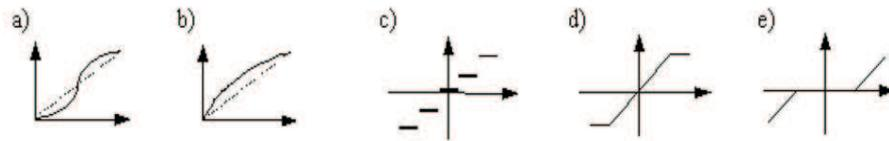
Fig. 1. Types of nonlinearity in the input-output characteristics of converters: smooth – a,b, with discontinuities – c,d,e.
