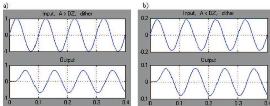
Fig. 6. Input and output signal of converter with dither  $D_{pp} = 0.4$ ,  $-0.2 \leq DZ \leq 0.2$ , a)  $A = 1$ , b)  $A = 0.18$ .
