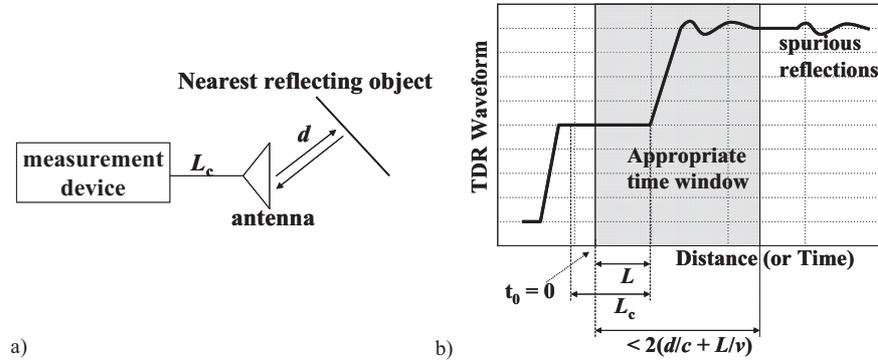
Fig. 2. Schematization of possible interferences from the environment a), and of the corresponding TDR waveform b).
