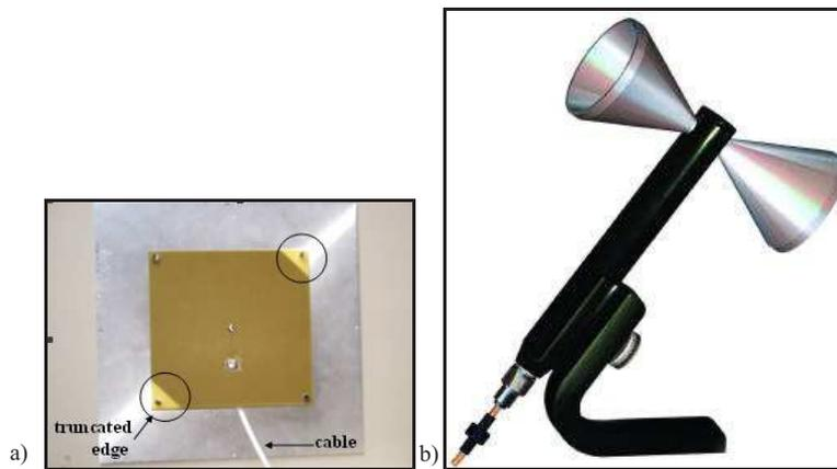
Fig. 1. RFID-reader antenna a), and biconical antenna b).
