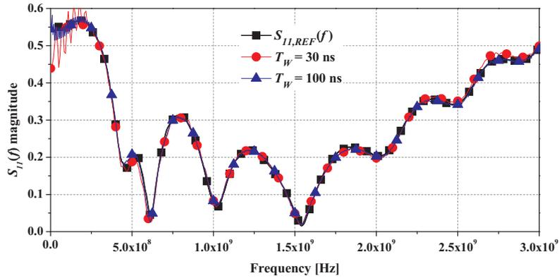
Fig. 7. Comparison between  $S_{11,REF}(f)$  and the  $S_{11}(f)$  curves obtained from FD-transformed data for different time windows ( $T_W$ ), for the biconical antenna.
