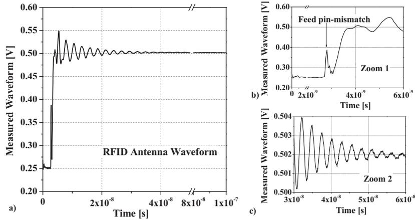
Fig. 3. TDR waveform of the RFID antenna for a 100 ns-long time window a), zoom of the initial portion of the waveform b), zoom of the noise-corrupted multiple reflection at longer times c).
