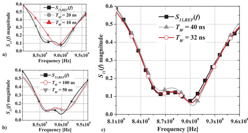
Fig. 4. Comparison between  $S_{11,REF}(f)$  and the  $S_{11}(f)$  curves obtained from FD-transformed data for different time windows ( $T_W$ ), for the RFID antenna.
