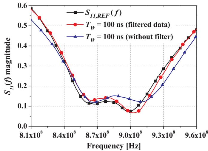
Fig. 5. Comparison between the  $S_{11}(f)$  derived from the FD-transformation on a 100 ns-long acquisition window with and without the application of a moving average digital filter.
