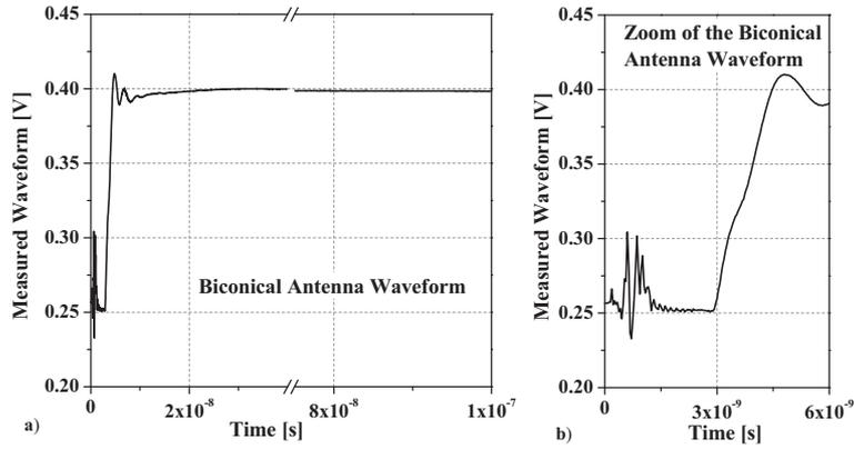
Fig. 6. TDR waveform of the biconical antenna for a 100 ns-long time window a), zoom of the initial portion of the waveform b).
