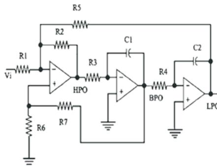
Fig. 1. Benchmark circuit (Continuous-Time State-Variable Filter).
