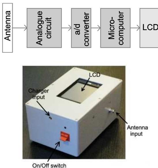
Fig. 1. Block diagram and photograph of GLOP2 locator.
