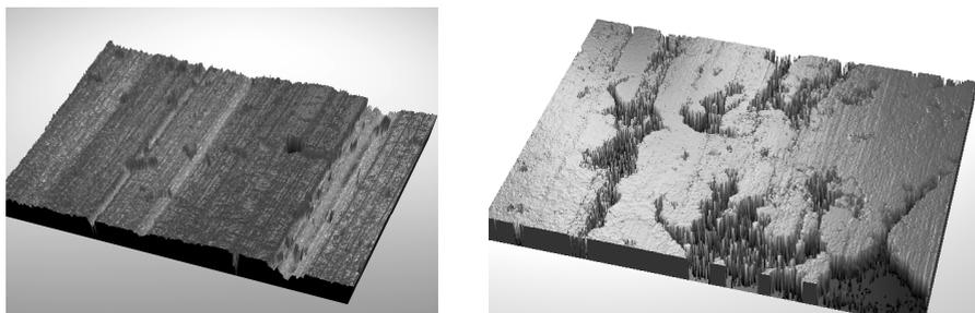
Fig. 5. Brake drum (left) and lining (right) after 250 000 kilometres of covered distance.
