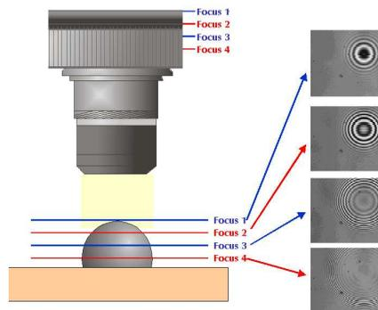
Fig. 3. Principle of vertical scanning in interferometry.
