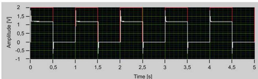
Fig. 7. Wave form of signal across the skin-electrode interface circuit in response to a square stimulus signal.
