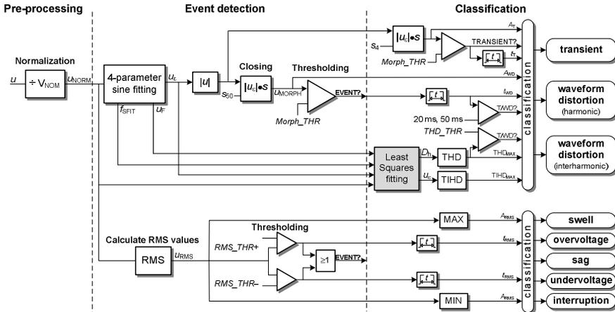
Fig. 2. Block diagram of the algorithms implemented in the PQ analyzer.
