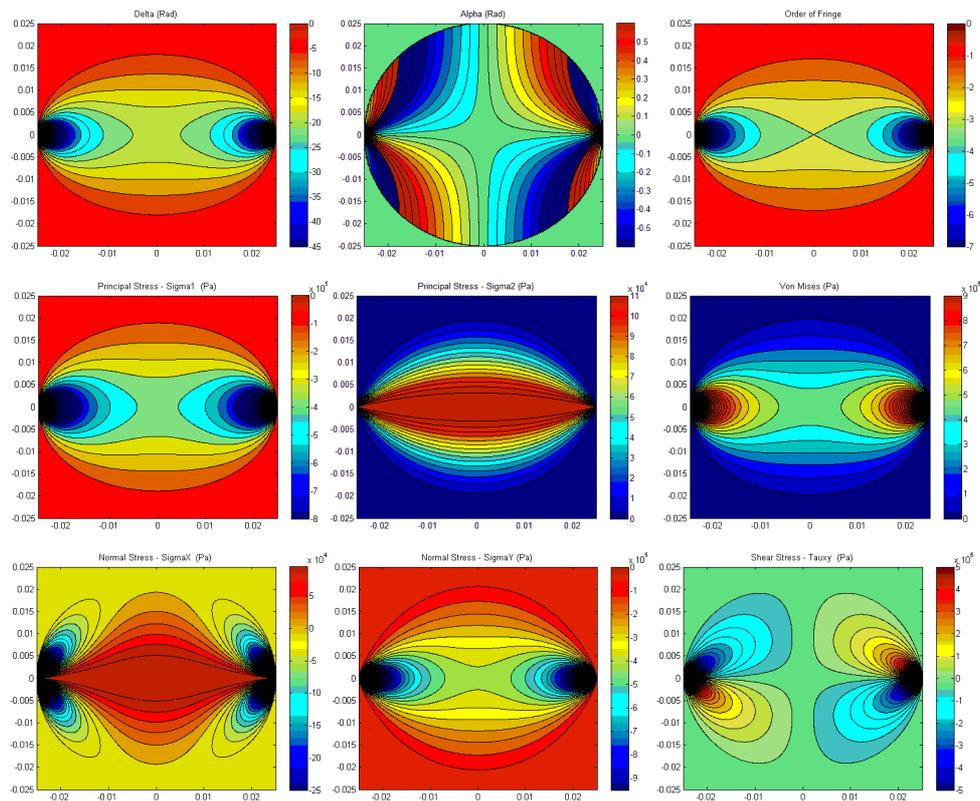
Fig. 4: Results obtained through experimental measurements using the new equations with  $N = 19$  and  $Step = 10$  of:  $\delta$ ,  $\alpha$ , fringe order( $n$ ),  $\sigma_1$ ,  $\sigma_2$ , von Mises stress( $\sigma_v$ ),  $\sigma_x$ ,  $\sigma_y$  and  $\tau_{xy}$ .
