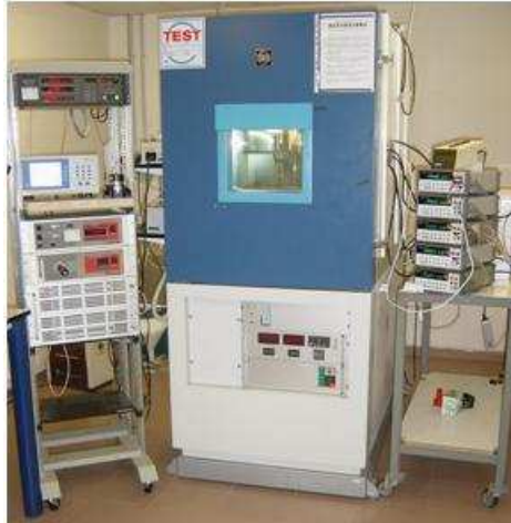
Fig. 4. The reference climatic chamber selected for the MID tests.
