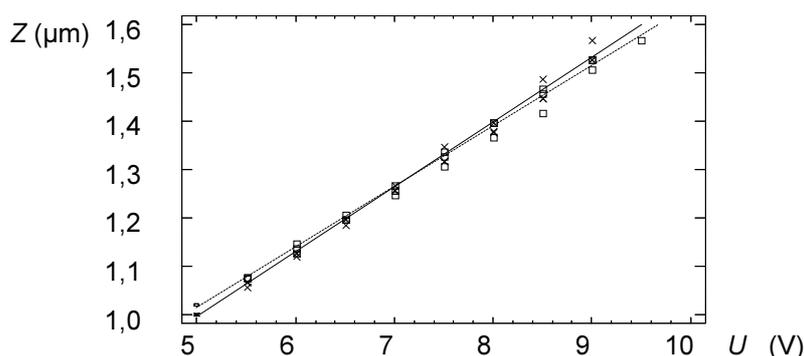
Fig. 4. Deflection of the plate's axis versus voltage for both directions of the deformation.
