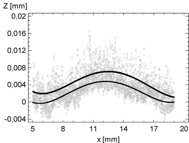
Fig. 2. The deformation of the piezoelement for voltages of 5 and 15V.
