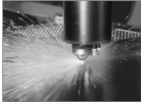
Fig. 3. Cutting bores with a laser cutter
